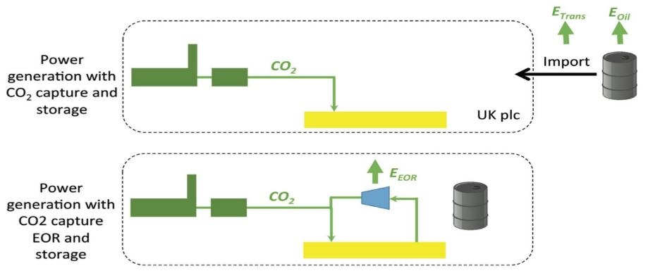
Compare emissions 3.96 Mt CO<sub>2</sub> of CCS plus imported oil against 4.25 Mt CO<sub>2</sub> emissions CCS + CO2-EOR which produces oil
